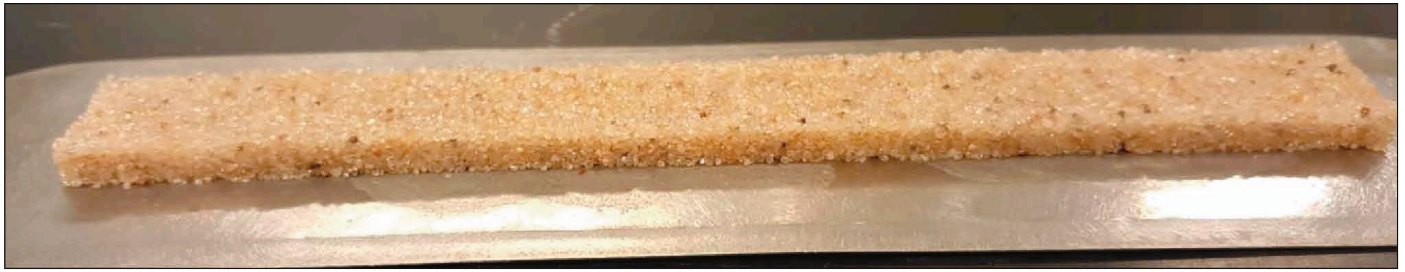
Fig. 1. A resin cured 20/40-mesh local sand pillar loaded on a conductivity measurement slab.
