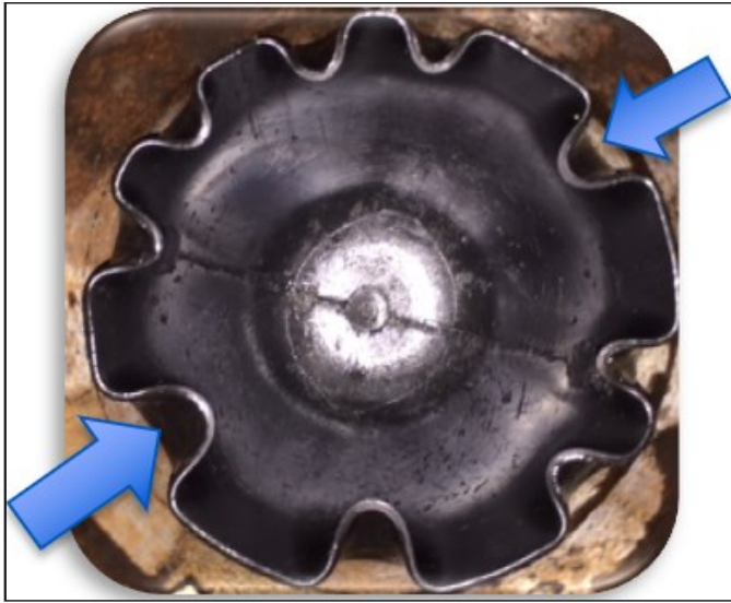
Fig. 3. Representing the flowing effect on the drillpipe wiper.
